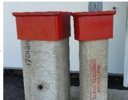
**Choose the correct driving cap for your machine** For a drop hammer, thumper style, use the ACP Driving caps. For a percussion style, pneumatic, vibrating style driver, you will need a manufactured driving head for your specific machine. ACP Driving Cap is **NOT** designed to be used with a percussion driver.
