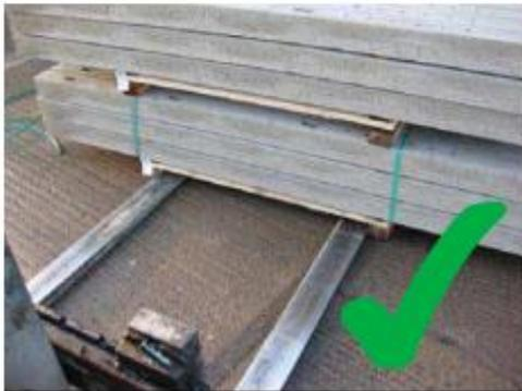
The forks must be widened to be as close to the load bearer as possible
