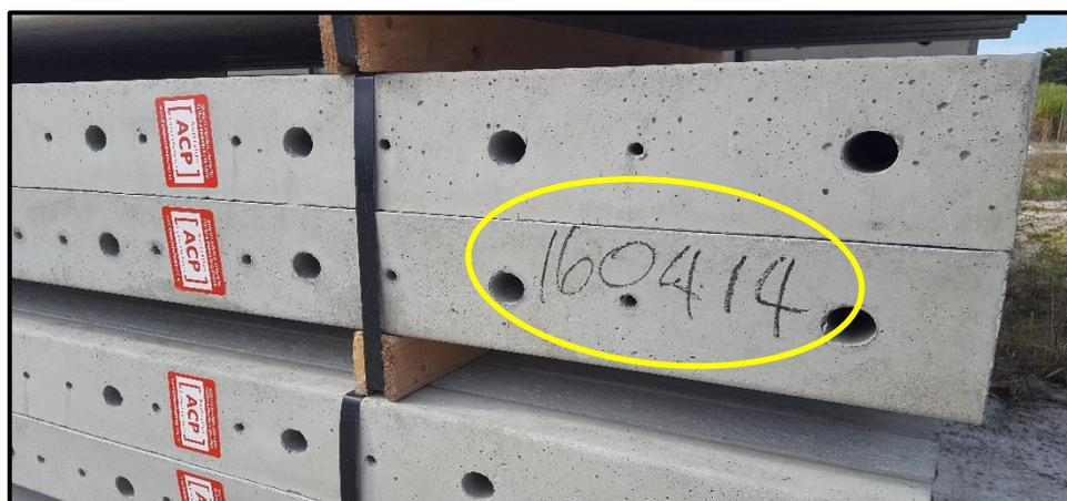
**ACP GUIDE: ALLOW 28 DAYS FROM DATE OF MANUFACTURE BEFORE DRIVING, HAMMERING, OR TENSIONING WIRE ON [ACP] POSTS.**
