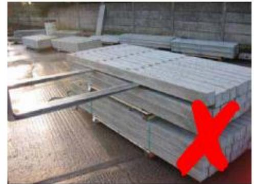
Products must not be taken out of packs using the forklift, they will damage the unit
