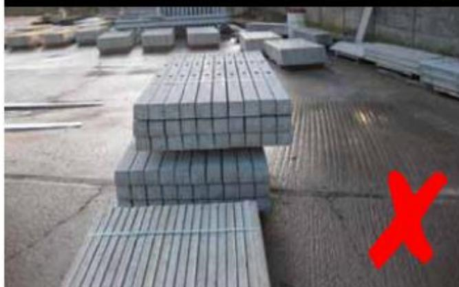
Products must not be stacked on top of each other like this as the load bearers are not in line
